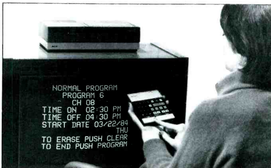
With this VCR, on-screen graphics guide the user through the programming sequence step-by-step.
